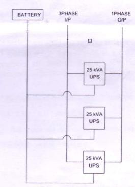
Parallel redundant / Modular UPS System
