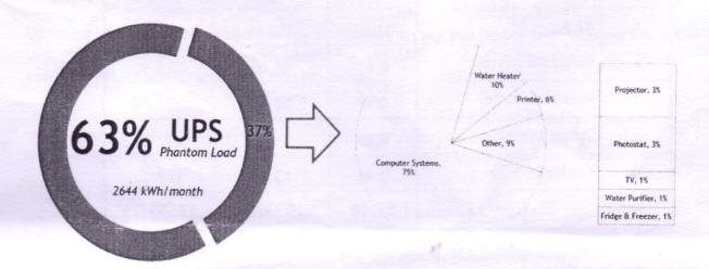
63% of the phantom load is contributed by the UPS System which is a necessity and cannot be eliminated but by proper optimisation we can minimise the phantom losses of UPS system. Whereas remaining 37% contributed by other equipment can be eliminated by simply turning them off when not in use.
