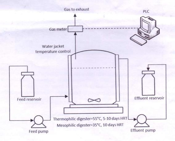
2 Stage High Performances Anaerobic Digester
